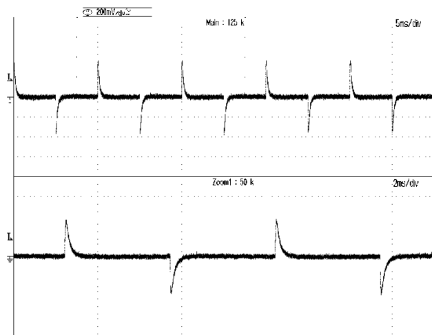
Figure 23: Output voltage response to step-change in load current (50%-75%-50% of full load; di/dt = 0.1A/\mu s ). Trace: Vout; 500mV/div; Time: 2ms/div
